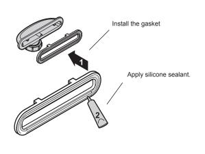
4. Attach the overflow mounting plate.
